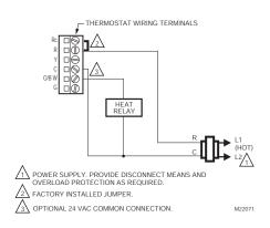
Fig. 9. Typical hookup of heat only system.
