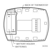
Fig. 14. Installing batteries.
