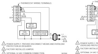
Fig. 6. Typical hookup of conventional 1H/1C system with one transformer.
