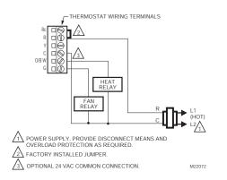
Fig. 10. Typical hookup of heat only system with fan.
