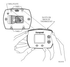
Fig. 15. Mount thermostat to wallplate.
