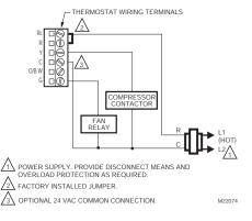
Fig. 12. Typical hookup of cool only system.
