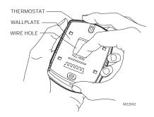
Fig. 2. Separate wallplate from thermostat.
