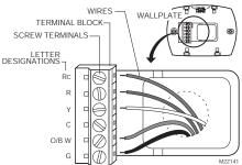
Fig. 5. Restrict wires to shaded area of wire hole.
