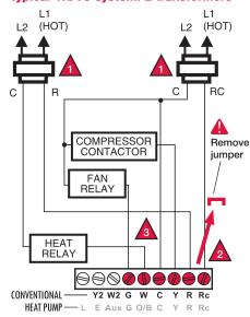
A Power supply. Provide disconnect means and overload protection as required.
