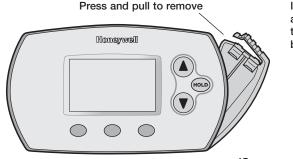
Insert fresh AA alkaline batteries, then reinstall battery holder
