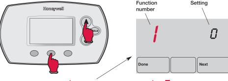
To begin, <u>press and hold</u> the ▲ and FAN buttons until the display changes
