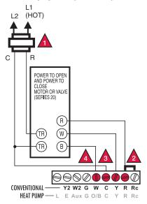
A Power supply. Provide disconnect means and overload protection as required.
