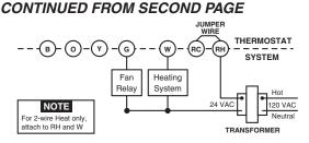
Figure 2. Typical wiring diagram for heat only, 3-wire, single transformer systems
