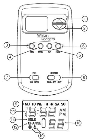
Figure 8. Thermostat display, buttons and switches
